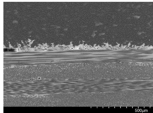
**Fig. 2-Interface region in a CFRP overmoulded specimen**
