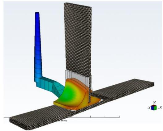
**Fig. 1-Flow simulation for a composite overmoulding case**
