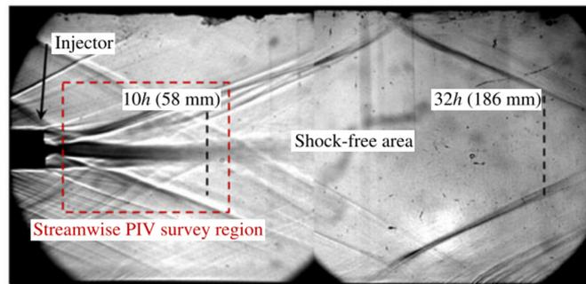
b) Schlieren of the test section
