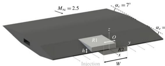
a) Strut injector equipped with expansion ramps
